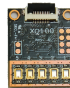
Ultra-compact 5 element QCM odor imaging sensor chip
