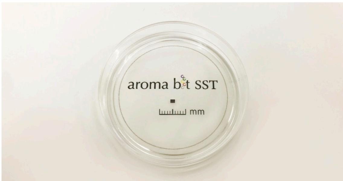
Chart4: Picture of 1mm squared die of silicon CMOS based smell sensor, with dog nose equivalent ~1,200 sensor pixels
