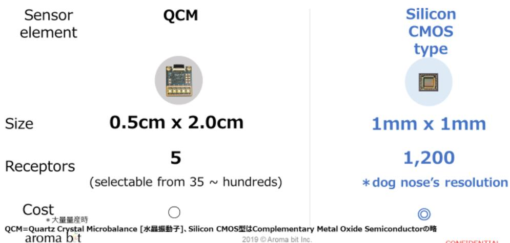
Chart 2: Comparison of the Odor Sensor elements of Aroma Bit(QCM type and the silicon CMOS type released now)
